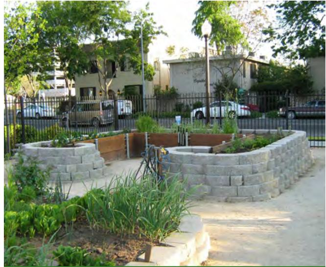
**Figure 3.1. Compacted, decomposed granite surfacing provides accessibility to the garden beds.** *Photo courtesy of City of Sacramento Department of Parks and Recreation*
